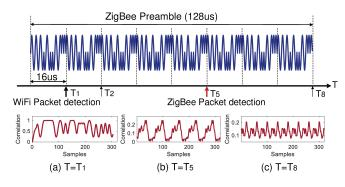
Fig. 7: Diagram of ZigBee preamble detection
