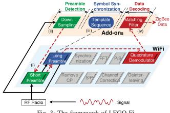
Fig. 3: The framework of LEGO-Fi
