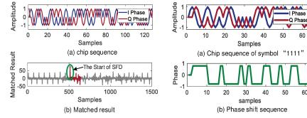
Fig. 6: Carrier frequency shift sequence (take symbol "1111" as an example)
