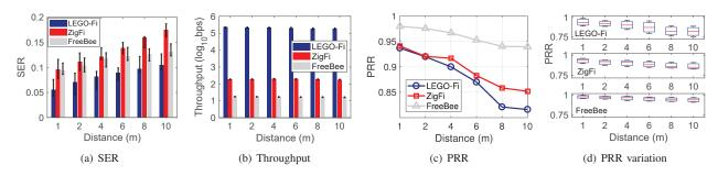
Fig. 14: Performance comparison with different distances between the ZigBee sender and the WiFi receiver
